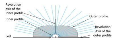
•Inner profile curve for maximum spacing between poles
