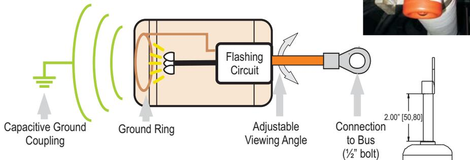
Capacitive coupling between the R-1VH / R-1VL and earth ground provides a means of completing the flashing circuit without a hardwired ground connection. This allows for enough energy to flash the LEDs.
